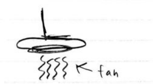
Figure 4: The hovercraft design is more of a imaginative concept than a practical one. In this design, a large propeller fan in the bottom of the structure to elevate the the wheelchair and another turnable propeller fan in the back of the structure to move the wheelchair in the desired direction.
