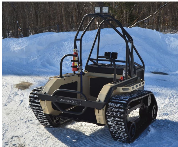
Figure 4: Ripchair 3.0. This track design was evaluated as this device performs very well in all terrains. [10]
