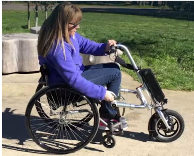
Figure 6: Firefly Electric Handcycle. This attachment can be fitted to an existing wheelchair to increase mobility. [12]
