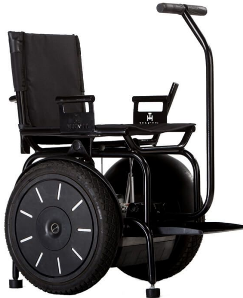
Figure 5: BLUMIL i2 seated segway. The segway is cheaper and less complex than the tracked solutions, but must be designed such that it is stable and versatile in various terrains. [11]
