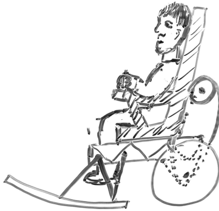
Figure 10. Sled concept sketch. The use of sleds in our design will aid in the traversing of soft or more fluent terrains. This includes sand and snow. The device will not exclusively have sleds and requires driving wheels in the rear. However, sleds offer a cheap way to conquer terrains and effectively replace casters or thin wheelchair wheels which fail in these terrains.
