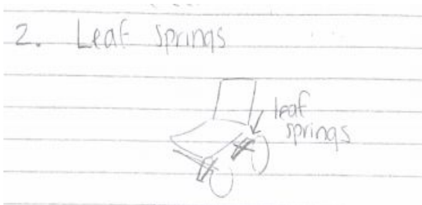
Figure 10: These are a cheap and effective way to damp our device when on rough terrains
