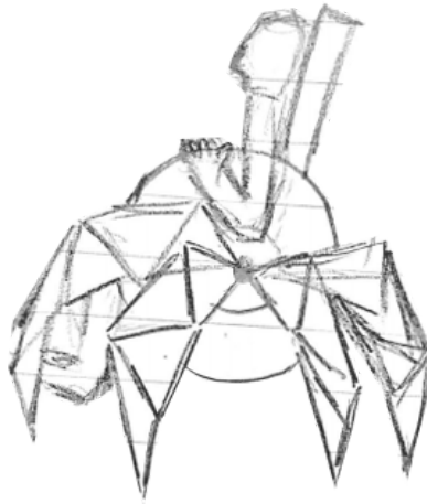
Figure 11. Mechanical legs concept sketch. This design utilizes the Jansen linkage that acts as “legs” of the wheelchair. The user then mechanically walks by the implementation of three sets of linkages mounted on either side of the user allowing them to move through soft terrains and step over obstacles.
