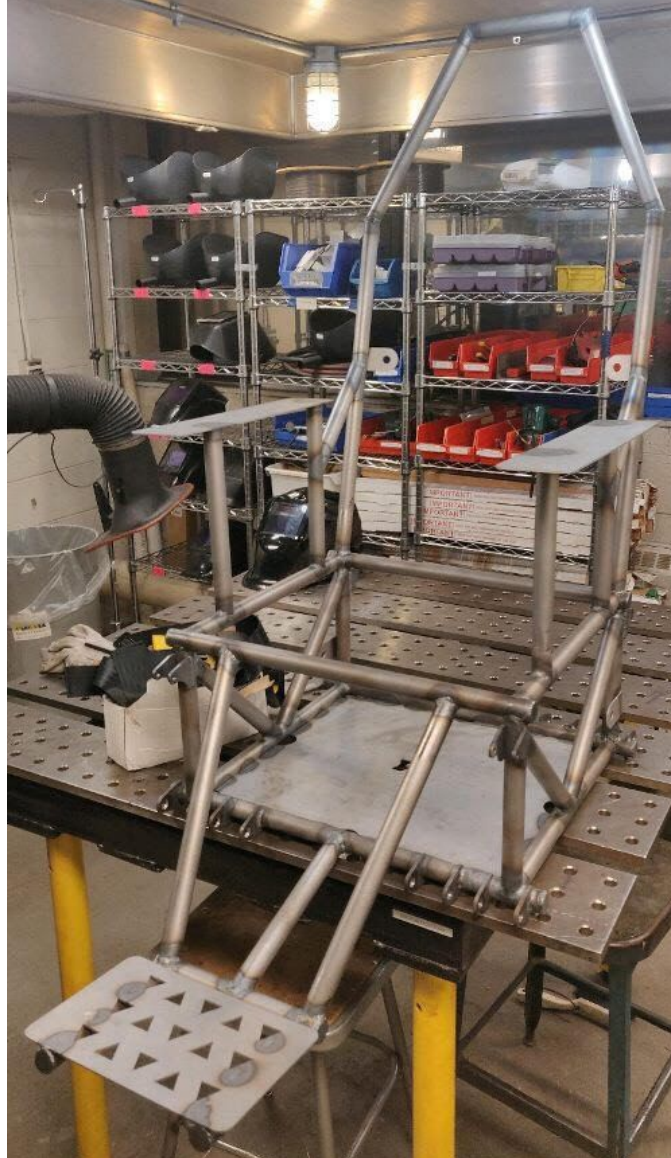
Figure 43. Human machine interfaces changes included the addition of a roll bar, backrest structural support, and leg rest structural support.
