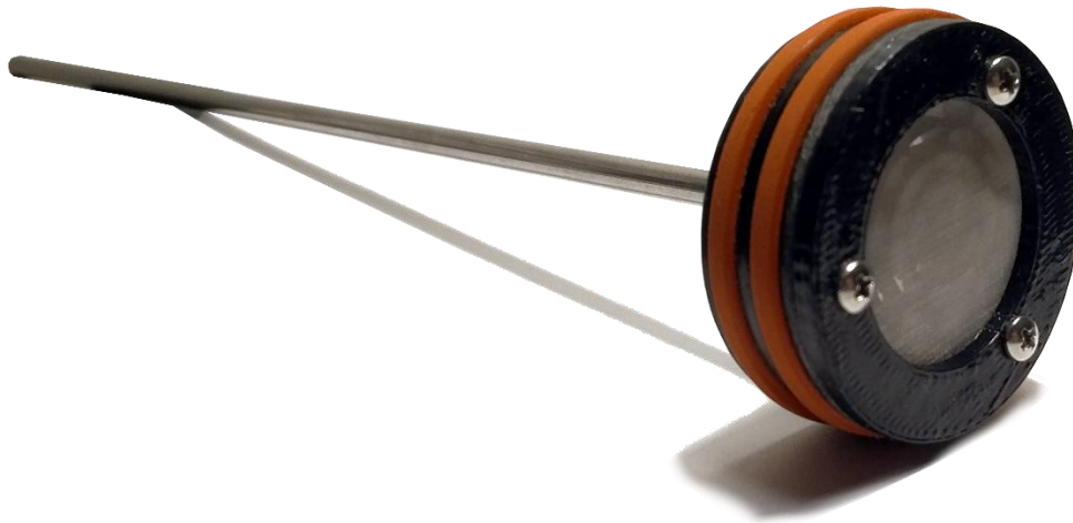
Figure 6) French press plunger which utilizes a steel mesh with 0.003" openings to filter out coffee grounds or tea leaves from the beverage. A double O-ring seal prevents leaks around the edges of the plunger.
