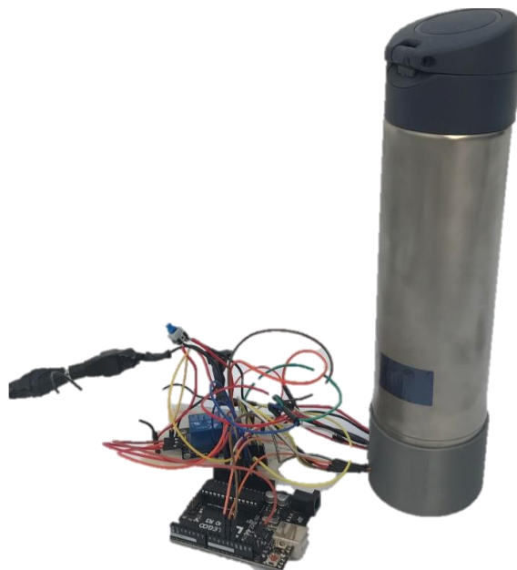
Figure 1) 1 st prototype Thettle created at the University of Michigan Makeathon. The electronic components were placed outside of the 3D printed housing below the thermos.
