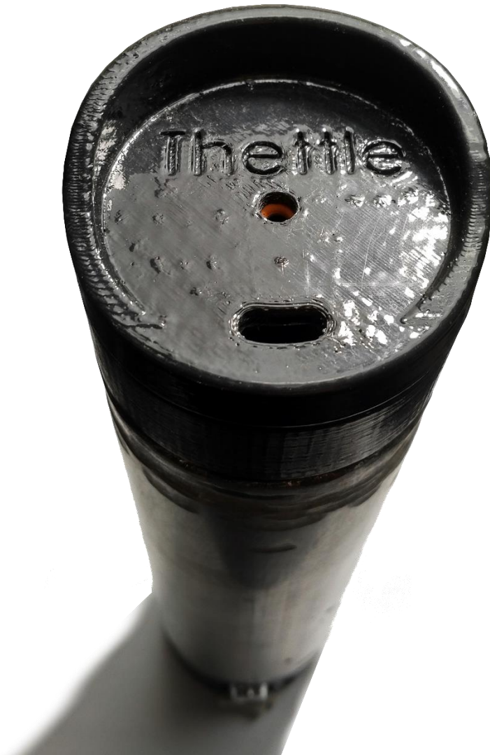
Figure 7) Lid of the thermos. It has a hole for the french press and an opening to drink out of. The lid rotates to close and uses O-rings to seal it.
